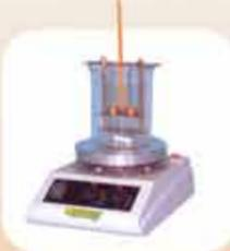
Ring and ball softening point apparatus
