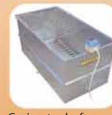
Curing tanks for concrete specimens
