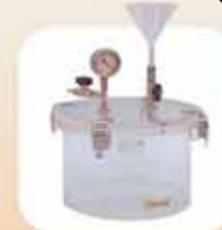
Vacuum pycnometer (rice test)
