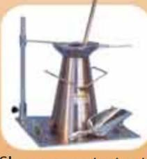
Slump cone test set
